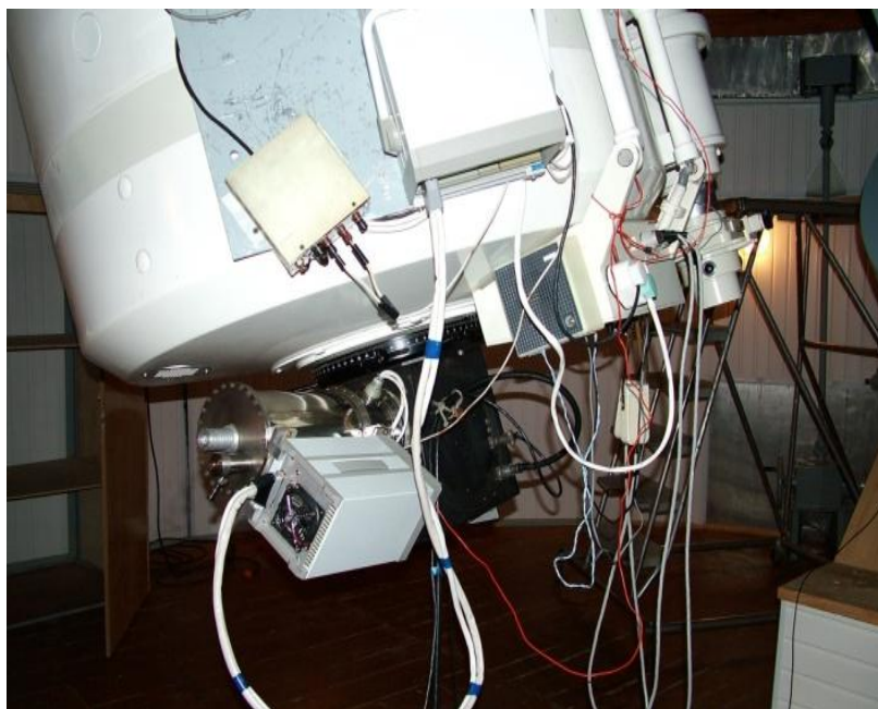
Fig6. Equipment of the 1m telescope: a CCD photometer with 2048x2048px by 13.5 microns. The field of view is 7'. The limit stellar magnitude is 23.5 mag. The medium-band photometry in UBVRI filters + narrow-band filters.
