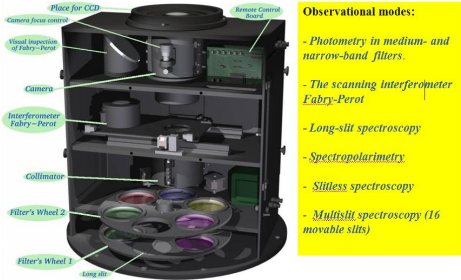
Fig2. Layout of the Spectral Camera with Optical Reducer for Photometrical and Interferometrical Observations (SCORPIO).
