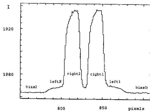
Figure 4: *The cross-section of the dispersion when the right circular polarization light is input.*
