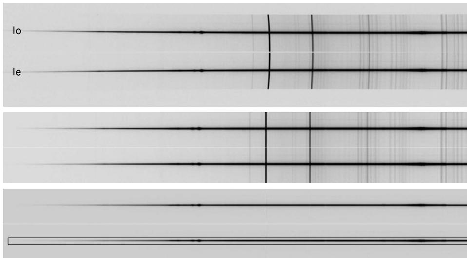
**Fig. 6.** Image processing with a single Wollaston prism: the top plot represents the original spectrum, the middle plot—the spectrum, corrected for the geometric distortions, and the bottom plot presents the spectrum after the background sky subtraction.
