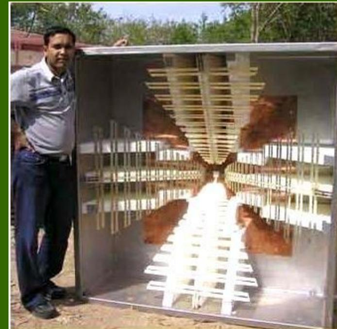
**FIG. 07 200 ÷ 800 MHz Eleven Feed for Giant Meter Radio Telescope.**
