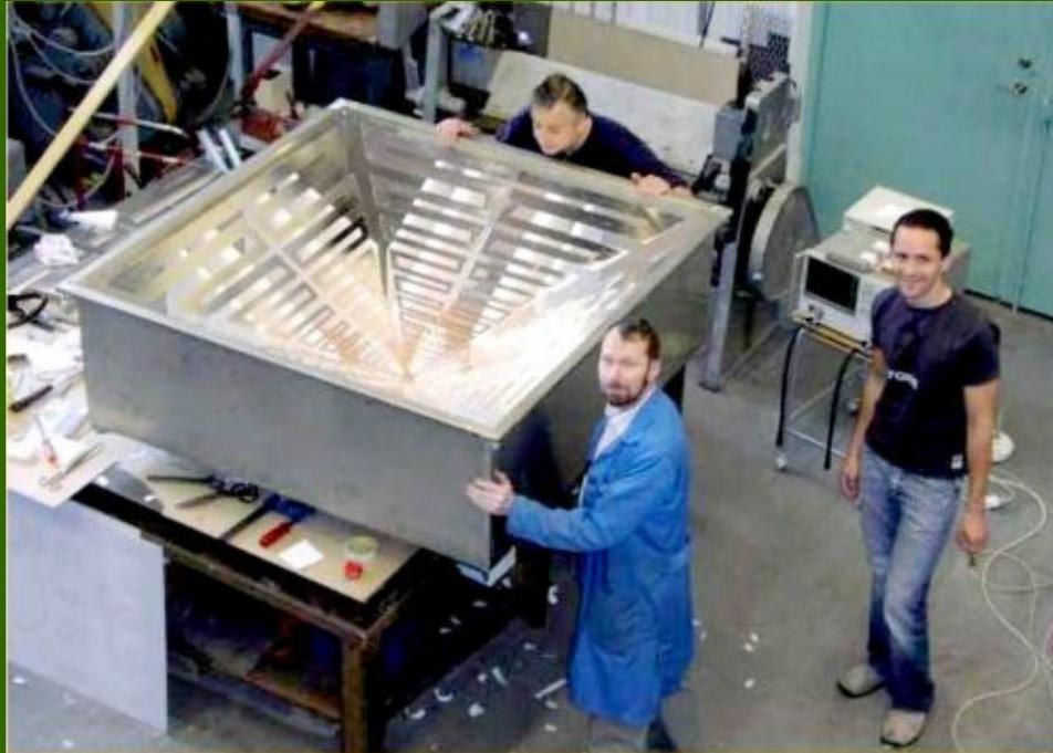
**FIG. 06 Mounting of 150 ÷ 2000 MHz Eleven feed for Green Bank Telescope in workshop at Chalmers. Developed for Caltech and MIT Lincoln lab.**
